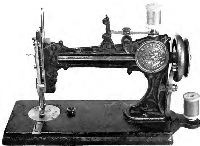
Figure 78.—CENTENNIAL SEWING MACHINE, 1876. The Centennial machine was basically a McLean and Hooper sewing machine which was renamed to take advantage of the coming Centennial celebration. It was based on the patents of J. N. McLean, March 30, 1869, and August 2, 1870, and made a two-thread chainstitch. Only about five hundred Centennial machines were manufactured in 1873, but by 1876 over three thousand had been constructed. The machines were advertised on white circulars which were printed in red and blue, and engraved with two women sewing, one by hand, labeled "Sewing in 1776," and one at a Centennial sewing machine, labeled "Sewing in 1876." There is no record that the machines were made after 1876. (Smithsonian photo 48216-T.)
